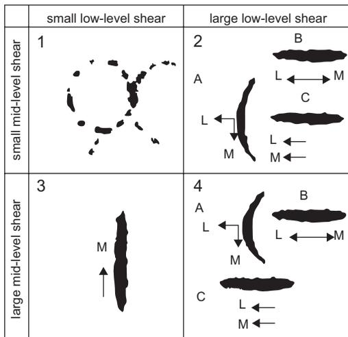
Fig. 11. Schematic depiction based in Lemone *et al.* (1988) and Johnson *et al.* (2005) of main categories of MCS convective organization for given vertical wind shear at low-level (0-2.5 km) and midlevel (2.5-6.0 km). Arrows marked L or M shows shear vectors for lower layer and middle one, respectively.
