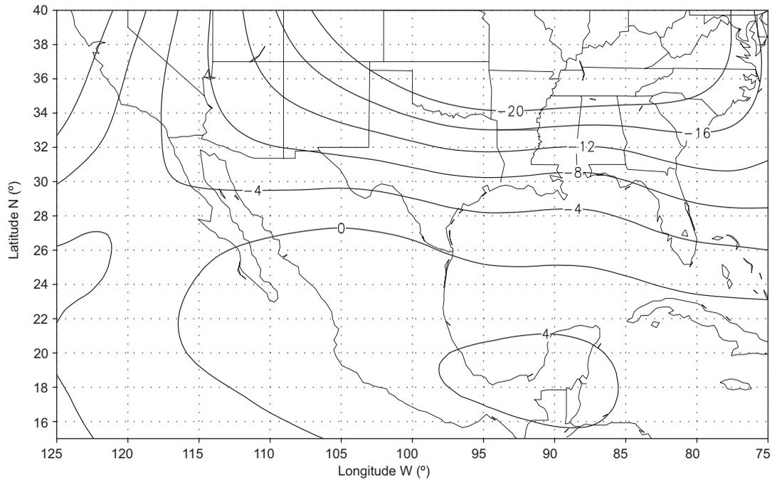
Fig. 2. 500 hPa heights (m) anomaly during July and August of 2004 from NOAA-NCEP Climate Diagnostic Center reanalysis data.
