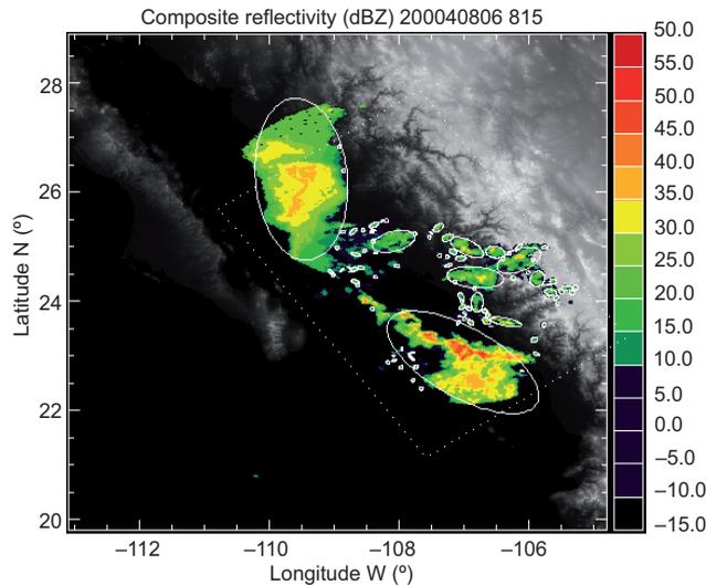
Fig. 12. Regional composite of radar reflectivity (dBZ) of the southern portion of NAME core region at 8:15 UTC August 6, 2004, which is showing a shear-parallel convective line, category 4C. Source: Colorado State University radar meteorology group.
