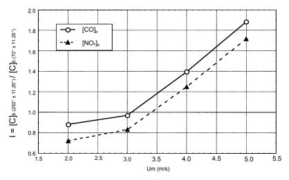
Fig. 3. Variation of the ratio between mean background concentration values  $I = [C]_{b(253^{\circ} \pm 11.25^{\circ})} / [C]_{b(73^{\circ} \pm 11.25^{\circ})}$  with mean ambient wind speed (Um).
