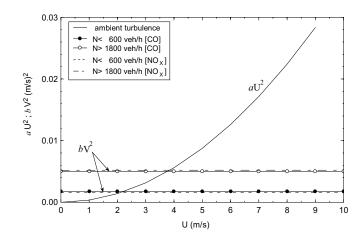
Fig. 16. Comparison of trafficinduced turbulence ( $\sigma_t^2 = bV^2$ ) for two traffic flow conditions (dashed and dotted lines) with ambient turbulence ( $\sigma_u^2 = aU^2$ ) for different wind speeds.
