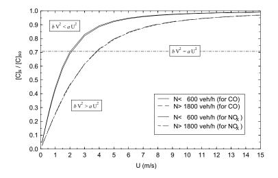
Fig. 14. Local concentration ratio between  $[C]_s$  (with traffic-induced turbulence) and  $[C]_{so}$  (without traffic-induced turbulence) versus wind speed for the two traffic flow considered. Leeward conditions.
