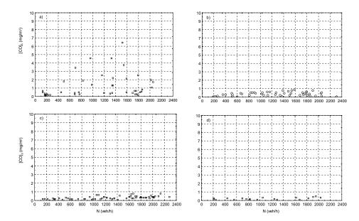
Fig. 6. Variation of  $[CO]_s$  with hourly traffic flow (N) for: a) U < 1.8 m/s, b)  $1.8 \le U < 3.0$  m/s, c)  $3.0 \le U \le 5.0$  m/s and d) 5.0 m/s < U. Windward conditions.
