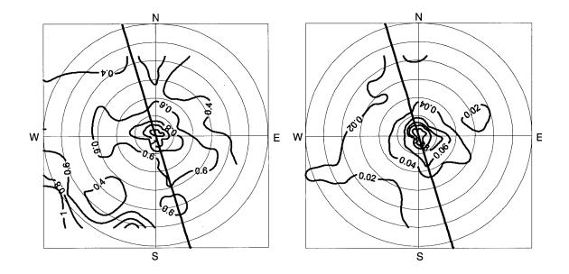
Fig. 1. Background pollution wind rose for CO. The central point represents calm winds while the concentric circles denote speeds at intervals of 2.0 m/s. The isopleths represent mean  $[CO]_b$  in mg/m<sup>3</sup>. The straight line indicates the orientation of the street canyon.
