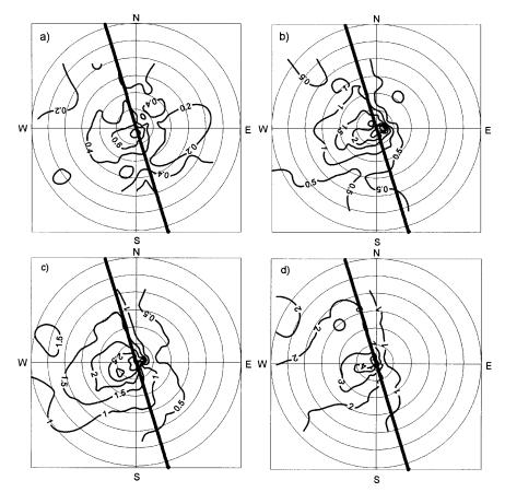
Fig. 4. Local pollution wind roses for CO considering different traffic flow: a) N < 600 veh/h, b) N: 600-1200 veh/h, c) N: 1200-1800 veh/h and d) N > 1800 veh/h. The central point represents calm winds while the concentric circles denote speeds at intervals of 2.0 m/s. The isopleths represent mean [CO]<sub>s</sub> in mg/m<sup>3</sup>. The straight line indicates the orientation of the street canyon.
