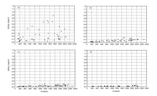
Fig. 7. Variation of  $[NO_x]_s$  with hourly traffic flow (N) for: a) U < 1.8 m/s, b)  $1.8 \le U < 3.0$  m/s, c)  $3.0 \le U \le 5.0$  m/s and d) 5.0 m/s < U. Windward conditions.
