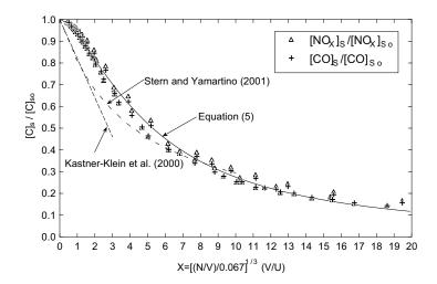
Fig. 15. Comparison of on site values of local concentration ratio between  $[C]_s$  (with traffic-induced turbulence) and  $[C]_{so}$  (without traffic-induced turbulence) and the fitted function (Eq.(5)) with wind tunnel (Kastner-Klein, 2000) and model simulation (Stern and Yamartino, 2001) results.
