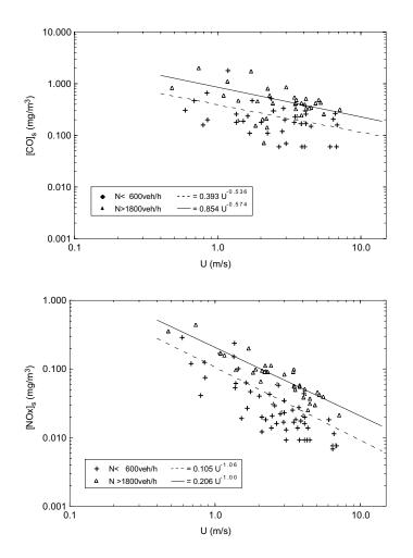
Fig. 8. Local CO concentration versus ambient wind speed for two traffic flows. Windward conditions.
