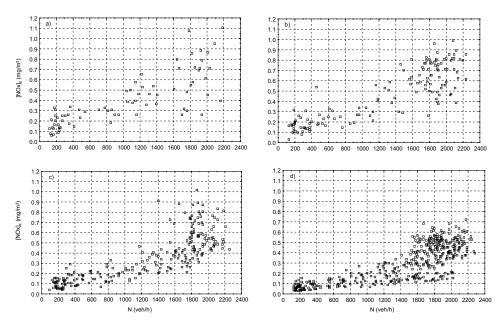
Figure 11. Variation of  $[NOx]_s$  with hourly traffic flow (N) for: a) U < 1.8m/s, b)  $1.8 \le U < 3.0$  m/s, c) 3.0 m/s  $\le U \le 5.0$  m/s and d) 5.0 m/s < U. Leeward conditions.
