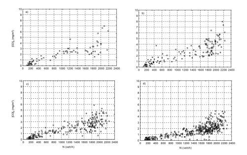
Fig. 10. Variation of  $[CO]_s$  with hourly traffic flow (N) for: a) U < 1.8 m/s, b)  $1.8 \le U < 3.0$  m/s c)  $3.0 \le U \le 5.0$  m/s and d) 5.0 m/s < U. Leeward conditions.
