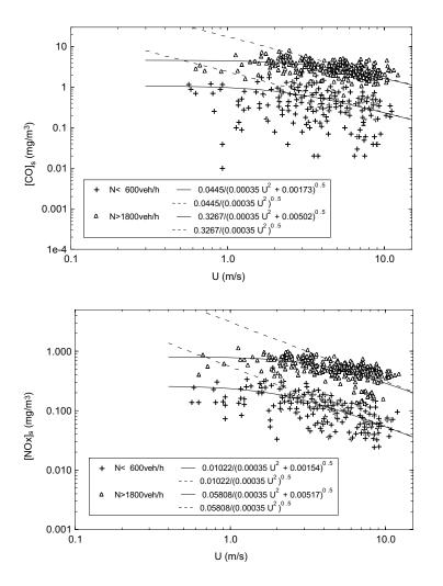
Fig. 12. Local CO concentration versus ambient wind speed for two traffic flows. Leeward conditions.
