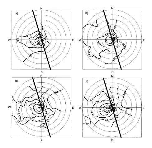
Fig. 5. Local pollution wind roses for NO<sub>x</sub> considering different traffic flow a) N < 600 veh/h, b) N: 600-1200 veh/h, c) N: 1200-1800 veh/h and d) N > 1800 veh/h. The central point represents calm winds while the concentric circles denote speeds at intervals of 2.0 m/s. The isopleths represent mean (NO<sub>x</sub>)<sub>s</sub> in mg/m<sup>3</sup>. The straight line indicates the orientation of the street canyon.
