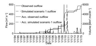
Fig. 16. Observed and simulated outflows (left *y*-axis) and observed and simulated accumulated outflows (right *y*-axis) for scenario 1 for the reservoir El Cuchillo from 1994 to 2014.
