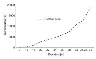
Fig. 2. Elevation of El Cuchillo reservoir vs. surface area (Huerta, 2015).
