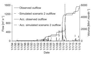
Fig. 17. Observed and simulated outflows (left *y*-axis) and observed and simulated accumulated outflows (right *y*-axis) for scenario 2 for the reservoir El Cuchillo from 1994 to 2014.
