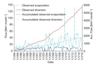
Fig. 3. Monthly simple and accumulated evaporation, as well as observed diversion in El Cuchillo reservoir from 1994 to 2014 (Conagua, 2014).
