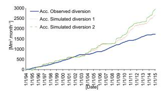
Fig. 11. Observed and simulated accumulated diversions for scenarios 1 and 2 for the reservoir El Cuchillo from 1994 to 2014.
