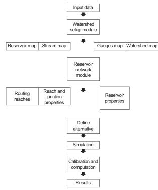
Fig. 5. ResSim modules, watershed setup, reservoir network and simulation (Alemaw et al., 2016).
