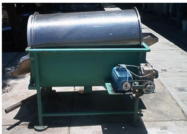
Fig. 1. View of pilot-scale cylindrical rotating screen for separation of vinasses flocculated solids
