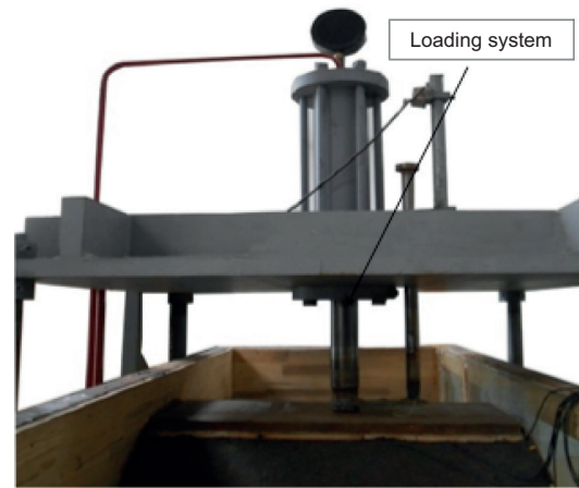
Fig. 1. The device of hydraulic loading.
