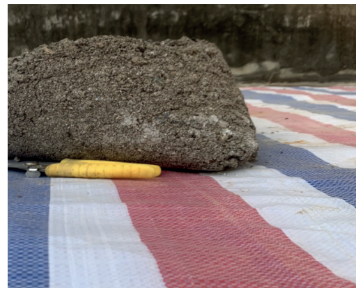
Fig. 12. IBA cemented into weak concrete blocks (Geotechnical toll for scale).
