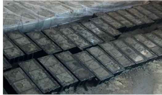
**Fig. 3.** Recovered steel fibers are embedded in the matrix.
