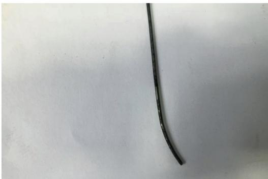
**Fig. 2.** Bent recycled steel fiber.
