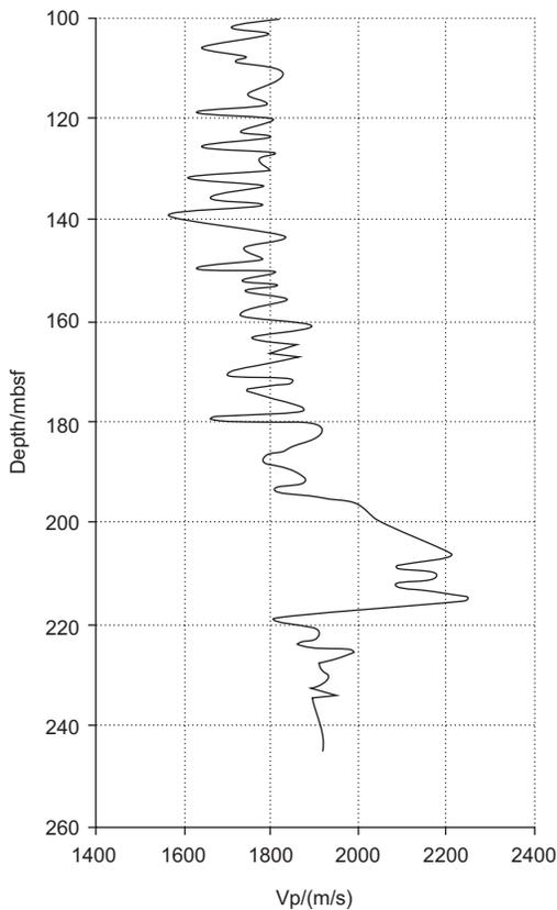
**Fig. 3.** The variation of P-wave velocity with depth in the well S.
