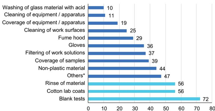
**Fig. 5.** Frequency of application of measures to control cross-contamination in sample processing. Other measures included keeping track of researchers' clothes colors, cleaning materials and hands with ethanol, and checking for particles by using microscopes in utensils prior to handling samples.
